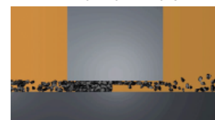
CONTAMINATION IN PRESENCE OF NARROW TOLERANCES
