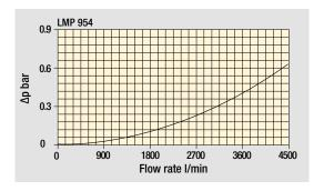
Pressure drop of filter complete with cartridge, oil viscosity 30 mm<sup>2</sup>/s (cSt)
