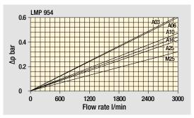
Bypass valve pressure drop
