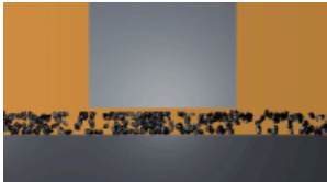
CONTAMINATION IN PRESENCE OF LARGE TOLERANCES
