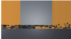
CONTAMINATION IN PRESENCE OF NARROW TOLERANCES
