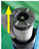
3 Remove the filter element
