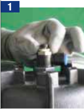
1 Loosen the air vent nut
