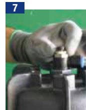
7 Make sure the air vent is closed
