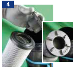
3 Insert the endcap with bypass or the possibly selected blind endcap in the filter element
