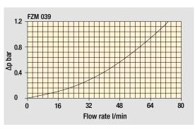
The curves are plotted using mineral oil with density of 0.86 kg/dm<sup>3</sup> in compliance with ISO 3968. Δp varies proportionally with density.
